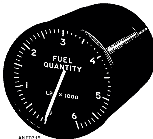
Figure 7-15.—Fuel quantity indicator.
