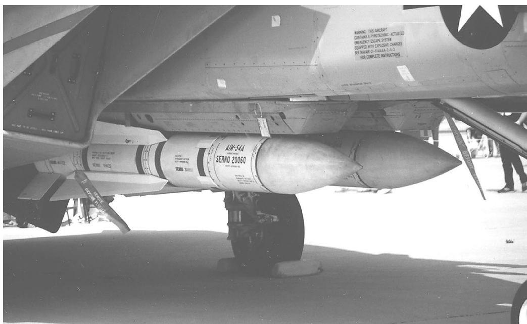
Figure 20-7.—Two AIM-54A Phoenix missiles mounted on the undercarriage of an F-14A Tomcat aircraft.
