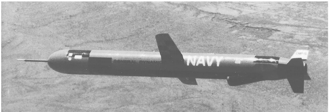
Figure 20-4.-The first fully guided Tomahawk cruise missile in flight after being launched from an A-6 Intruder aircraft.
