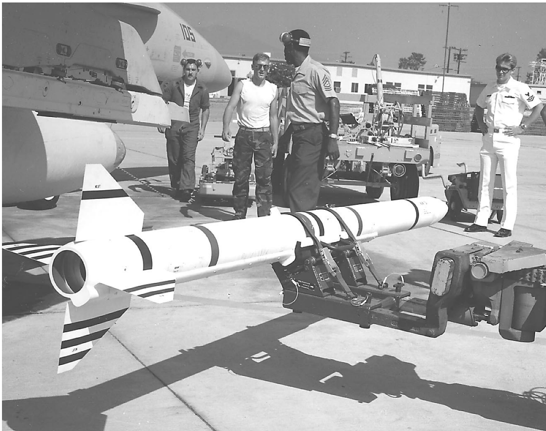
Figure 20-8.—An AIM-120A advanced medium-range air-to-air missile (AMRAAM) being readied for loading on an F/A-18A Hornet aircraft. 134.57
